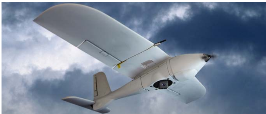
Figure 1 | The Desert Hawk hand-thrown UAS has a payload that warfighters can swap out just by removing a few bolts.
